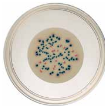
Figure 1. Thermo Scientific Chromogenic Coliform Agar (ISO) growing E. coli (pink to red) and coliform (dark blue/violet) colonies on membrane filter.
